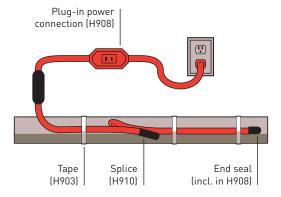
Table 5: Accessories for Raychem heating cable for pipe applications
